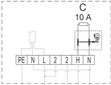
Fig. 14: Connecting electric heater (position C)
