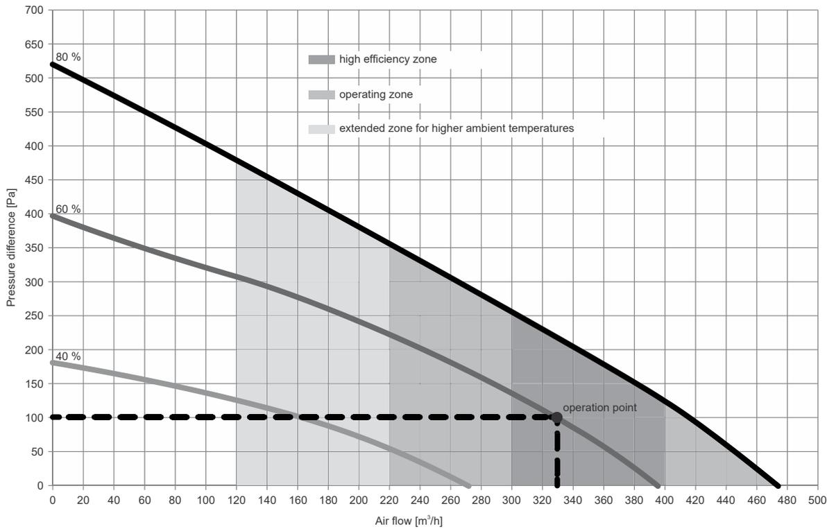
Fig. 4: Aerodynamic characteristic of the heat pump fan
