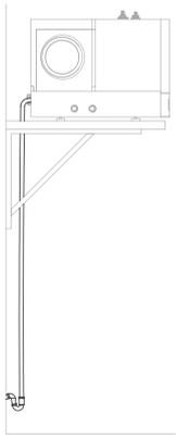
Fig. 6: Condensate drainage
