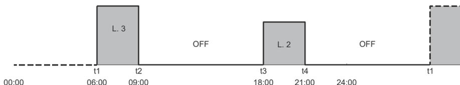
Fig. 11: Example of setting the timer – ventilation feature
