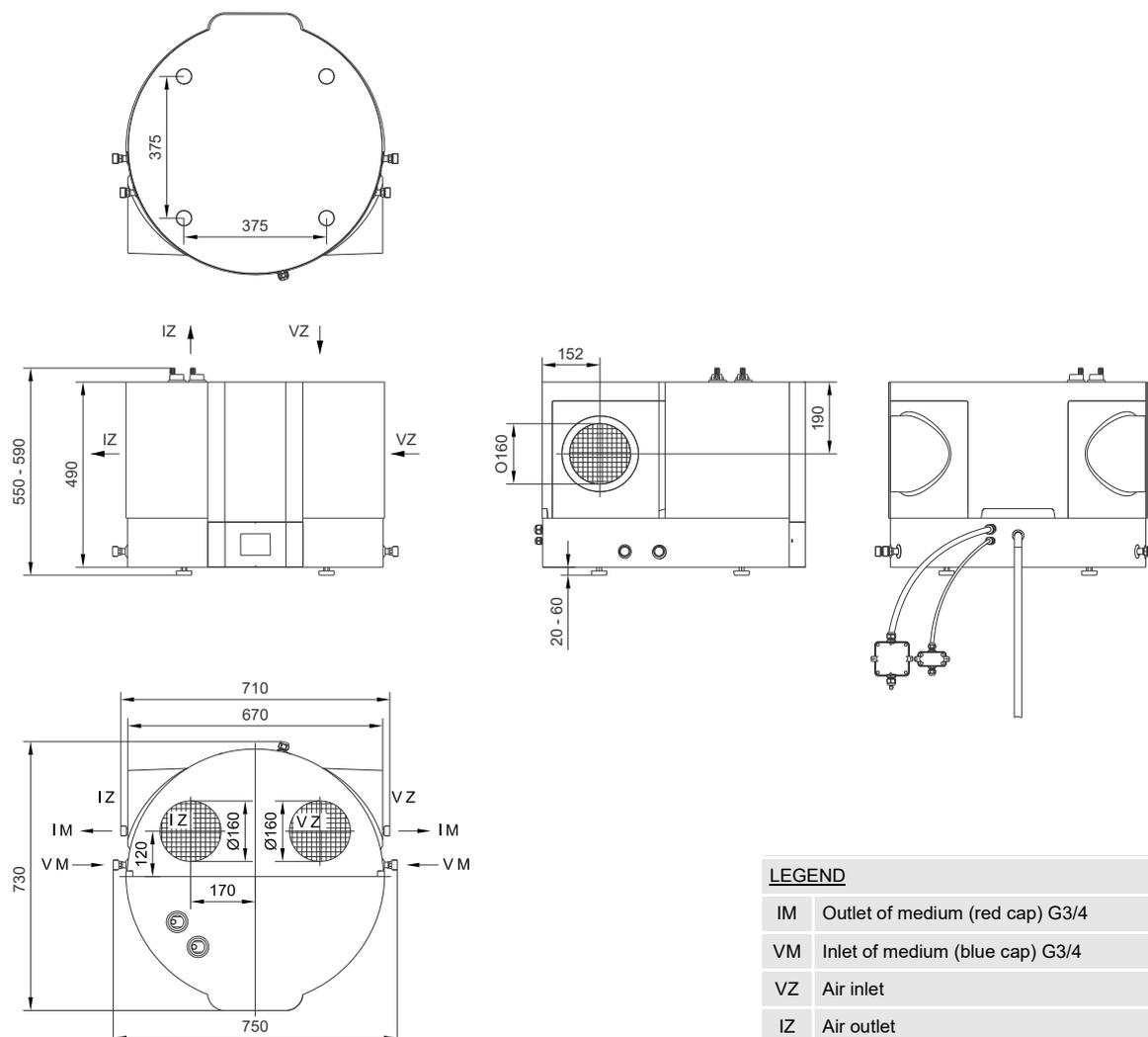
Fig. 1: Connection and installation dimensions of the heat pump [mm]
