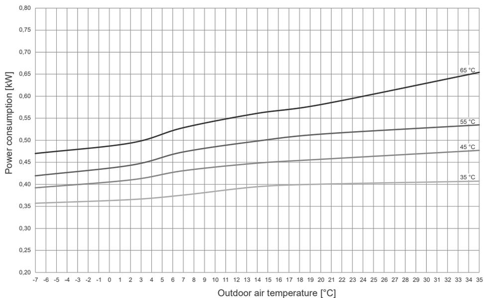
Diagram 2: Consumption of electrical power in accordance with EN14511
