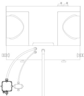
Fig. 12: Junction box for connecting external control of the "PV", "LT", "ECF" and "EHP" features
