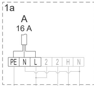
Fig. 8b: Connecting to power supply network (position A)
