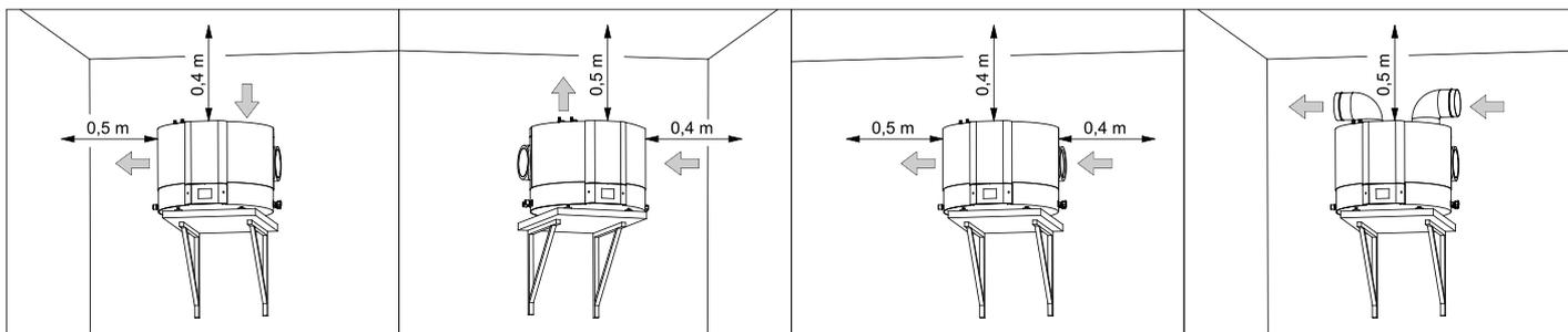
Fig. 2: Manners of use of suction and outlet openings
