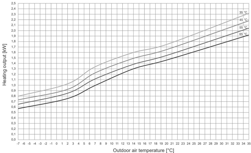
Diagram 1: Heating power in accordance with EN14511
