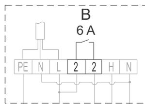
Fig. 13: Connection of a contact for controlling the "PV", "LT", "ECF" and "EHP" features
