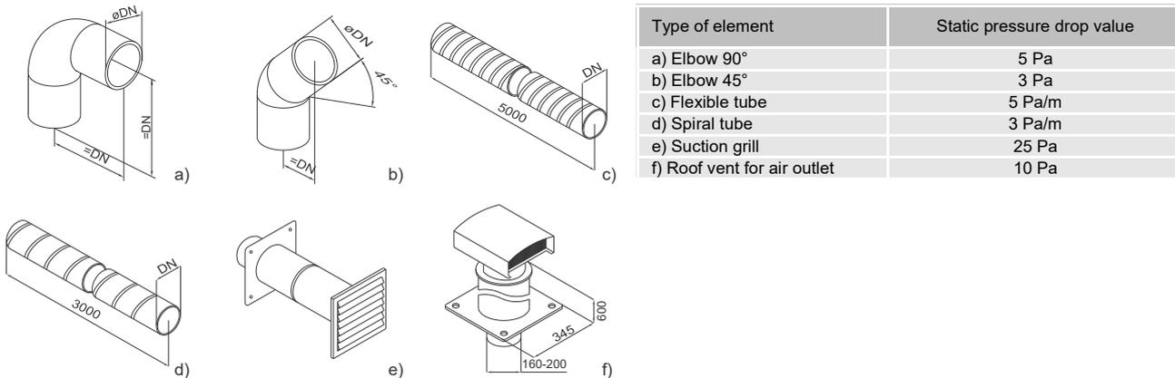
Fig. 5: Schematic demonstration of the basic elements in a pipeline system for inlet and outlet of air
