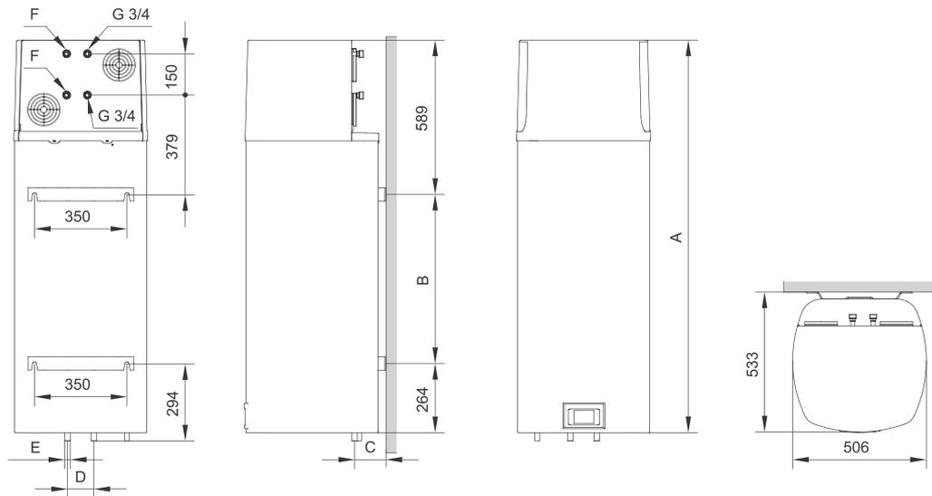
Fig. 2a: Connection and installation dimensions of the heat pump [mm]
